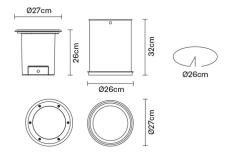
**Description** Downlight with anodized aluminium structure.
