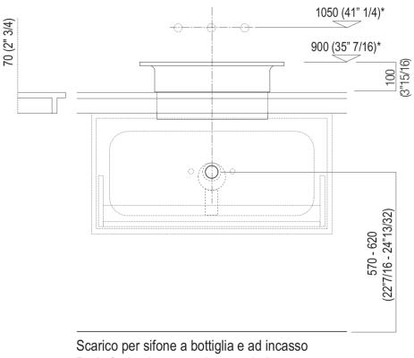
Drain for bottle trap and concealed waste trap
